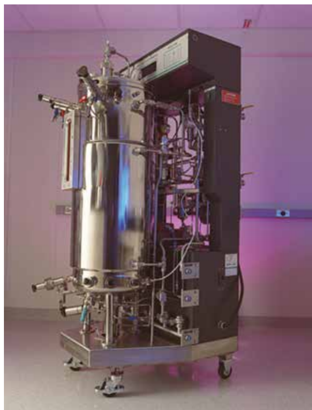
▲ Figure 5. This mobile pilot-plant fermenter has a 90-L capacity for the production of cellulosic ethanol. Source: U.S. Dept. of Energy.
